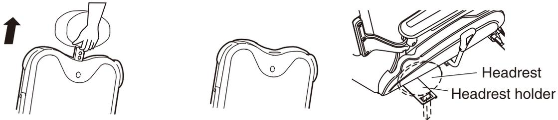
**CAUTION** When pulling out the headrest, be sure to ensure that metal fittings of the headrest do not hit the customer's head.
