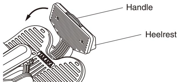
**CAUTION** Be sure to grasp the handle of the heelrest when moving the heelrest. Take care not to pinch foot of the customer or your finger in between the heelrest and step.
