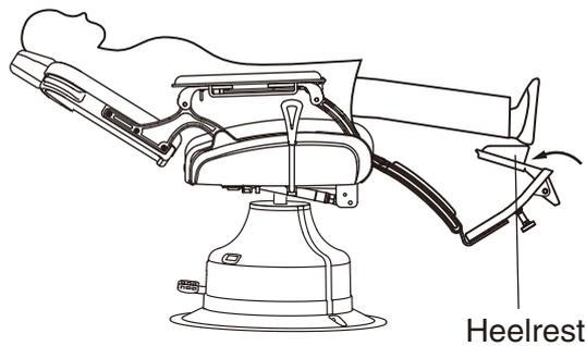
Grasp the handle of the heelrest when moving the heelrest.
