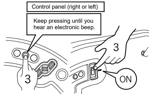
4. Setting is completed when the electronic beep is emitted. Return the chair to its original position by using the auto-return switch, and use the preset switch to check the set position.
