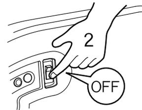
3. Press and hold the preset switch where you want to save the setting (P1, P2, or P3), and turn on the power switch. Keep pressing the preset switch for approximately three seconds.
