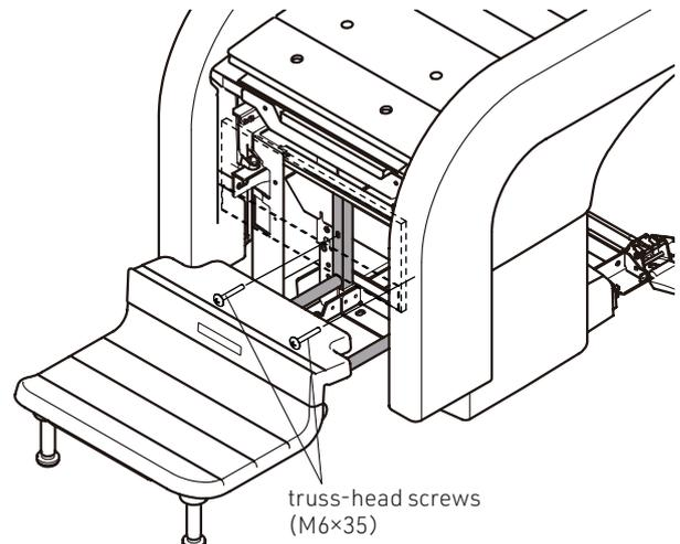
※If, in the procedure on the previous page, the bottom screw positions do not align, use the procedure below.
