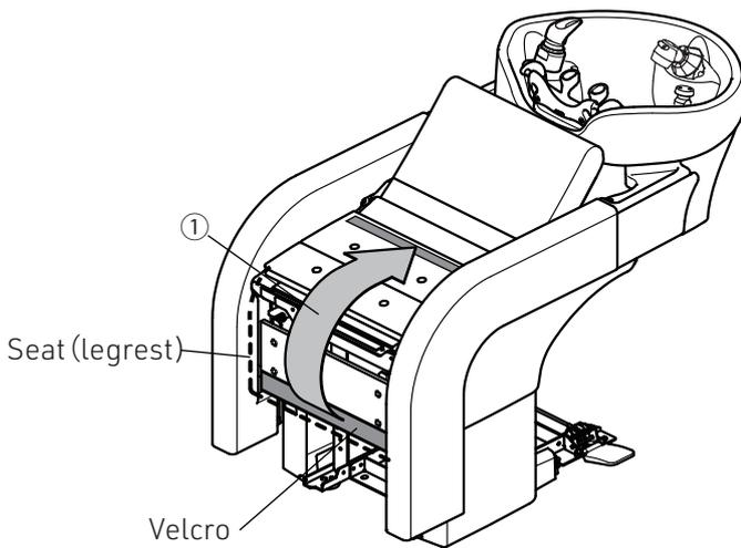
② Remove the front of the bottom protection mat from the seat frame to see the screw holes.
