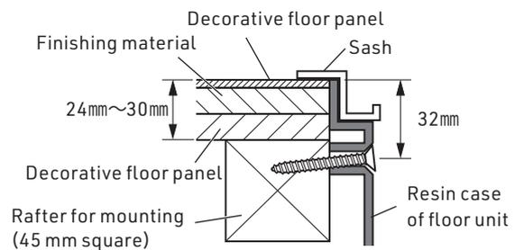
• Machine screws for use (packaged with floor unit)
