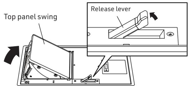
3. Hold the handle part of the top panel swing to open the top panel swing to right angle.
