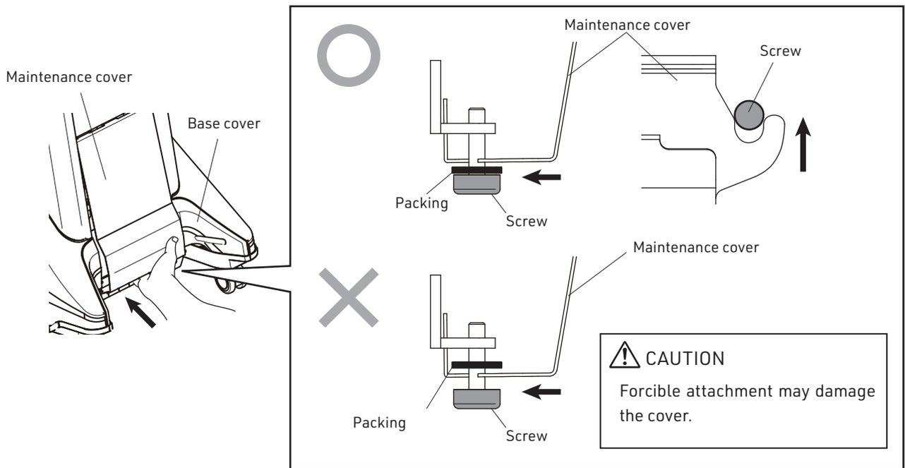
**CAUTION** When the maintenance cover is attached, pay attention not to hit the base cover. Forcible attachment may damage the cover.
