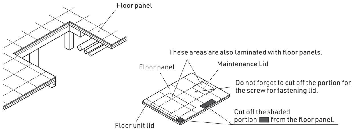
※Be sure to cut off in an exactly same shape as the cut window.
