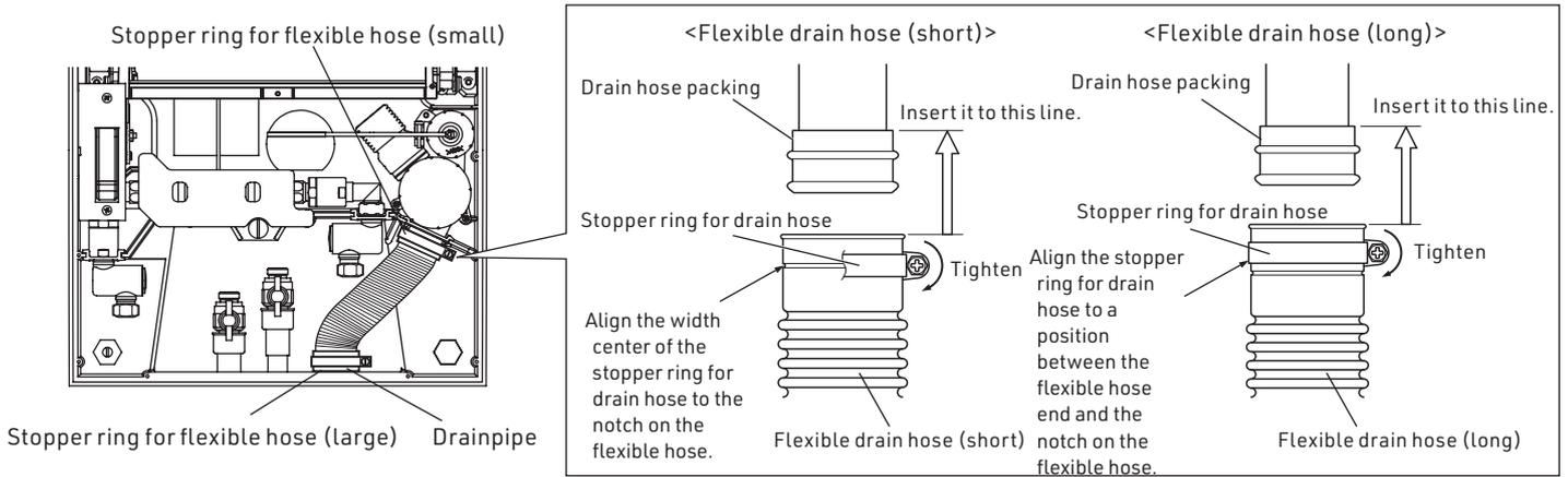
**CAUTION** The end of the drain trap is processed for prevention of the hose from slipping off. Ensure that the stopper ring for drain hose is not fastened over the thick end of the hose end. It may cause leakage.
