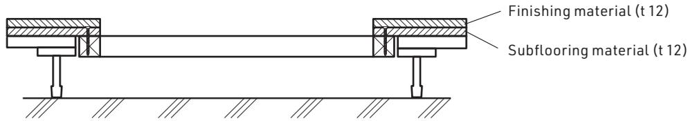
※ Check the flexural level of the floor base panel again and place additional support legs under the reinforcement frame if required.
