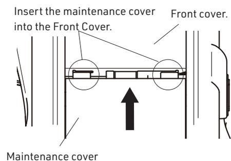
3. Make the bottom of the maintenance cover caught by the loosened screws.
