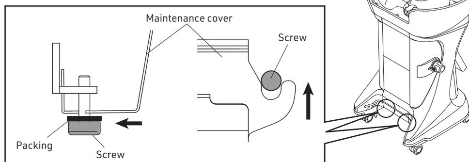
1. Loosen the screws (two positions: left and right)
