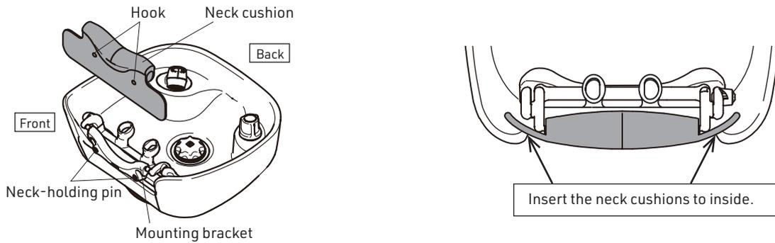
2. Attach the left hooks of the neck cushion to the neck-holding pins of the mounting bracket. (Check that both front and back hooks are attached.)
