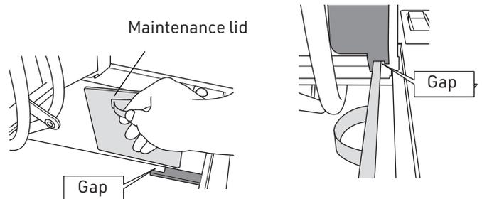
5. Hold the opening generated by removing the maintenance lid and lift the top panel upward.
