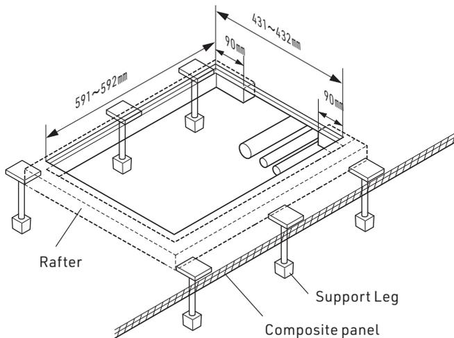
※ The adjustable range of floor unit is up to 150 mm from floor level.
