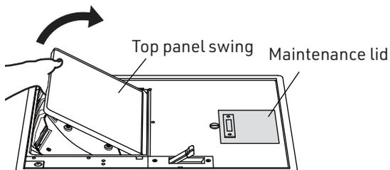
4. Remove the maintenance lid and insert it into the gap of the opened top panel swing.
