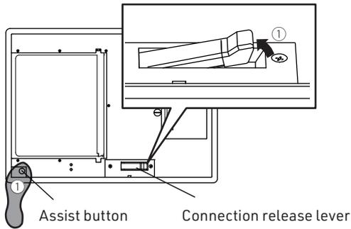
2. While the assist button is held down, use another foot to raise the release lever to the angle shown in the image. The top panel swing opens.
