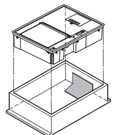
2. Install mortar filling so as to level the surface with the top end of the bury frame.
