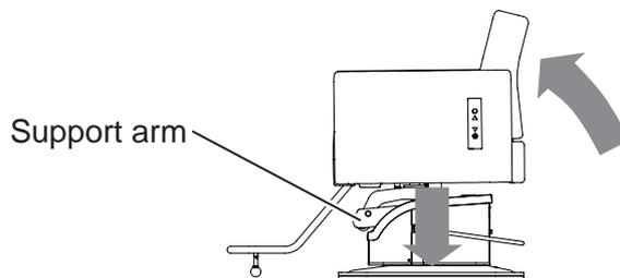
**Warning** When using the preset function or the auto return function, make sure that there is no human body, limbs, or objects in the gap between the chair or step or in the support arm, and operate it.
