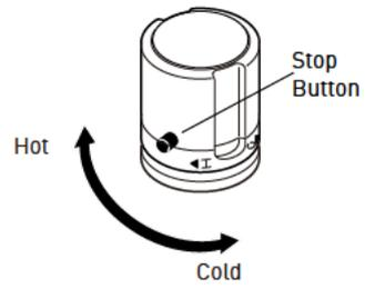
To adjust the temperature over 40 degrees, turn the knob while pressing the Stop Button
