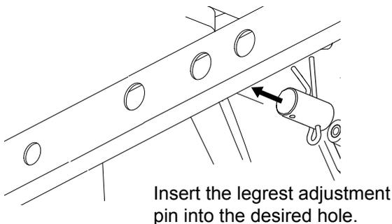
1. To set the legrest rising angle to Setting (1), insert the legrest adjustment pin into the Hole for Setting (1).
