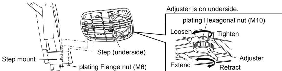
⇒The adjuster, which prevents the chair from overturning, is located on the underside of the step. To adjust the adjuster, loosen the plating hexagonal nut (M10) by using a wrench (No. 17) to adjust the height of the adjuster, and then tighten the plating hexagonal nut (M10) by using a wrench (No. 17).
