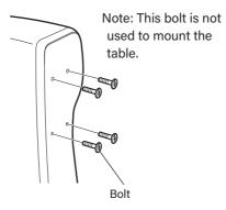
3 Attach the table bracket using the four hexagon head bolts (black) that have been provided.
