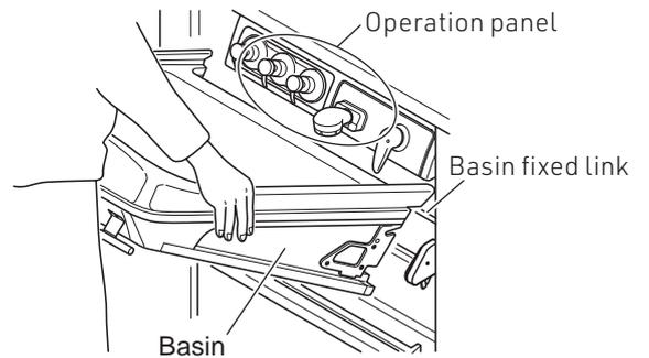
\* When the lever is set in the free position, lift the basin fixed link and turn the lever to the lock position.
