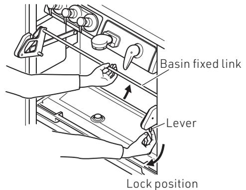
7 Insert the basin straight into the basin body parallel, with keeping the clearance between the basin and the operation panel.
