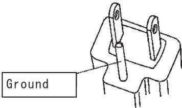
Failure to follow this instructions may cause electric shock if there is a malfunction or ground leakage. Contact a professional for grounding.
