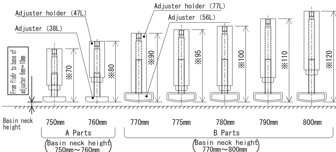
©The above ※value is just for reference. Please adjust the adjuster so the distance from floor to base of adjuster would be 6mm~10mm.
