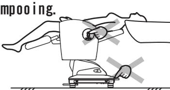
Take care not to accidentally operate the foot switch or manual switch, or trip over the foot switch or base part during shampooing a customer. Failure to follow this instruction may cause the unit to operate suddenly, leading to injury.
