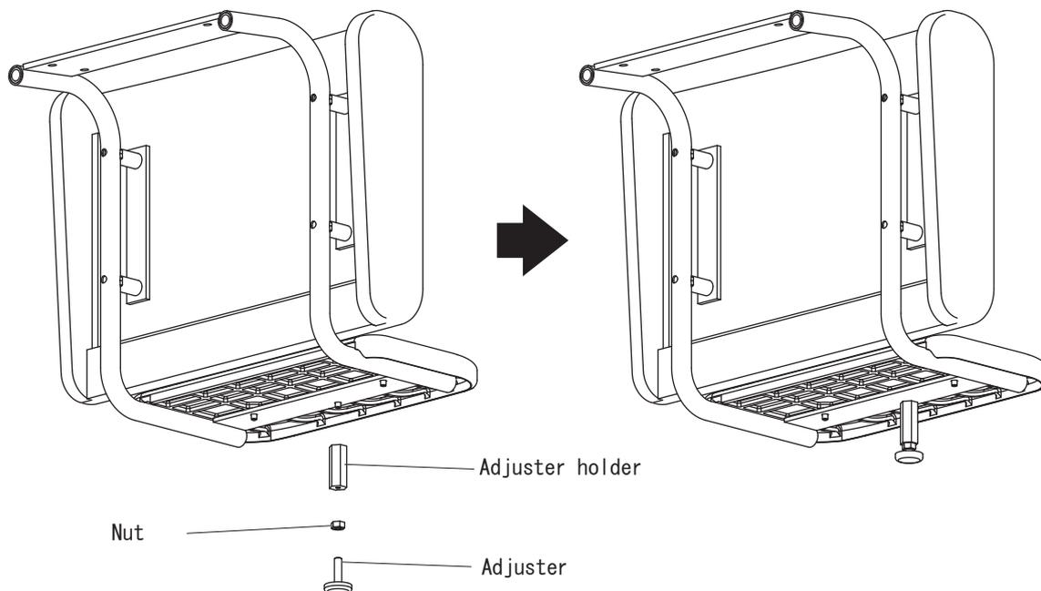
Attach the step adjuster as per the above illustration.
