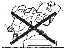
Do not get on or apply load to the legrest when it is in the raised position. Failure to follow this instruction may cause the chair to fall over, leading to injury, or damage the chair.
