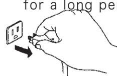
Remove the power plug if the product will not be used for a long period of time, such as after work or when the shop is closed. Dust and moisture may cause faulty insulation, leading to a ground leakage fire.
