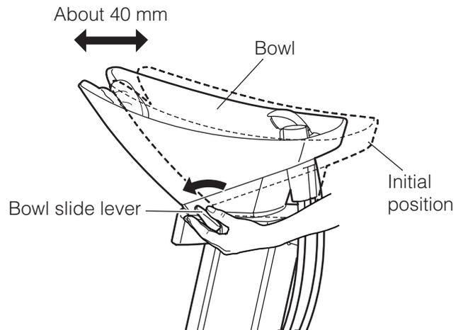
\* The bowl can be locked at four positions (including the initial position). The total sliding distance is about 40 mm.
