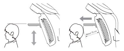
4 Alarm rings when the head position is misaligned
