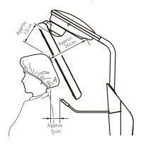
3 Setting the Roller Ball F in the correct position
