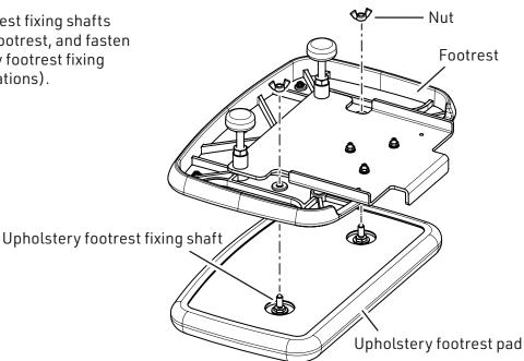
③ Fix the footrest onto the main unit, referring to 'Installing the Footrest' in the THE ONE Installation Instructions.
