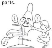
Long-term use may cause threads, nuts, bolts, etc., to become loose. Perform a monthly inspection on threaded parts to check for looseness. If any part is loose, tighten it firmly with a tool such as a screwdriver. If the part is still loose after retightening, please contact your local authorised Takara Belmont dealer.
