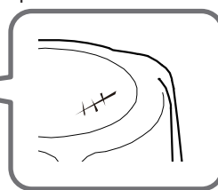
Example of a scratch on a plated surface
