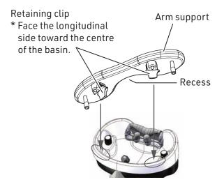
Place the retaining clips so that the longitudinal sides of the clips are at the centre of the basin, and press the arm support down from above to fit it.
